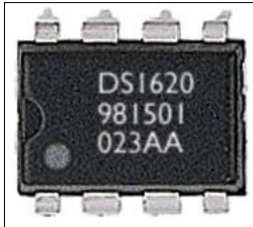
Figure 4: Digital Thermometer, DS1620
